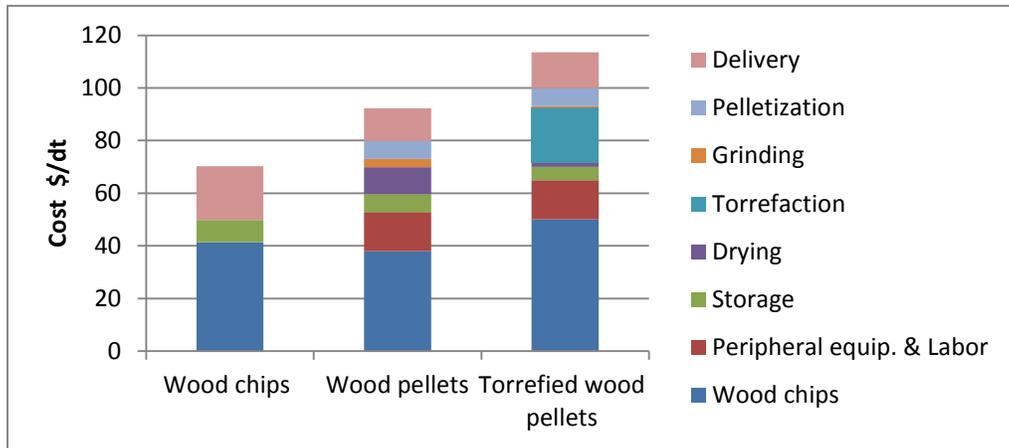
**Figure B2.19.** Costs of power plant feedstock of each scenario on a dry basis. Transportation cost is included as a distance of 100 miles is assumed. Poplar at a cost of \$41.33/dt was used as feedstock.
