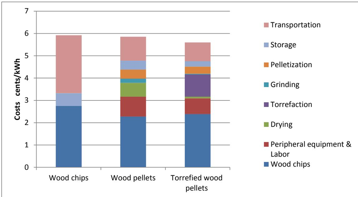
**Figure B2.17.** Cost contribution to electrical power generation from wood chips, wood pellets and torrefied wood pellets when a distance of 300 miles from the RBPD to the power plant is applied. Poplar was used as the feedstock at a biomass cost of \$41.33/dt.
