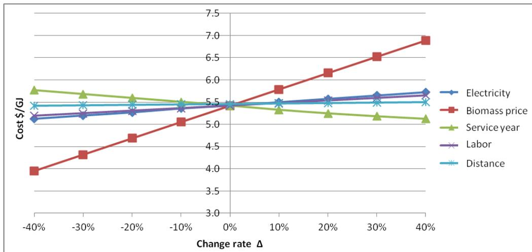
**Figure B2.20.** Sensitivity analysis for scenario 3: “Torrefied wood pellets.” Costs are in U.S. dollars per GJ of torrefied wood pellets.
