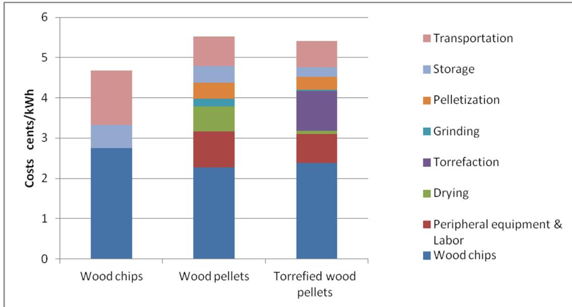
**Figure B2.16.** Cost contribution to electrical power generation from wood chips, wood pellets and torrefied wood pellets when a distance of 100 miles from the RBPD to the power plant is applied. Poplar was used as the feedstock at a biomass cost of \$41.33/dt.
