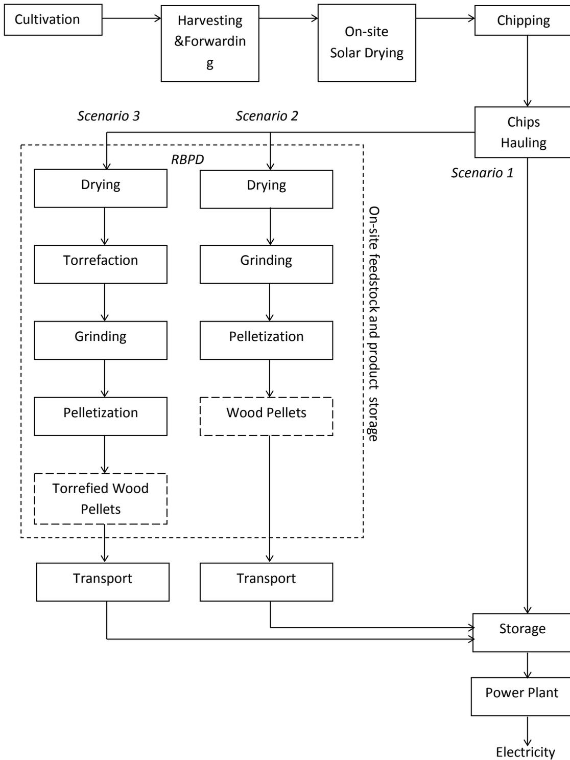
**Figure B2.13.** A depiction of the three systems being compared. 1) “Wood Chips” for direct co-firing at the power plant, 2) “Wood Pellets” with pelletization at RBPDs, and 3) “Torrefied Wood Pellets” with torrefaction and pelletization occurring at RBPDs.
