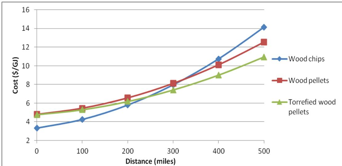
**Figure B2.18.** Cost comparison of the three scenarios at the power plant gate at varying transportation distance. Transport cost was calculated using a fixed cost of \$3.72/ton and a variable cost of \$0.074/ton-mile. An individual truck capacity of 40 tons was used for this analysis.
