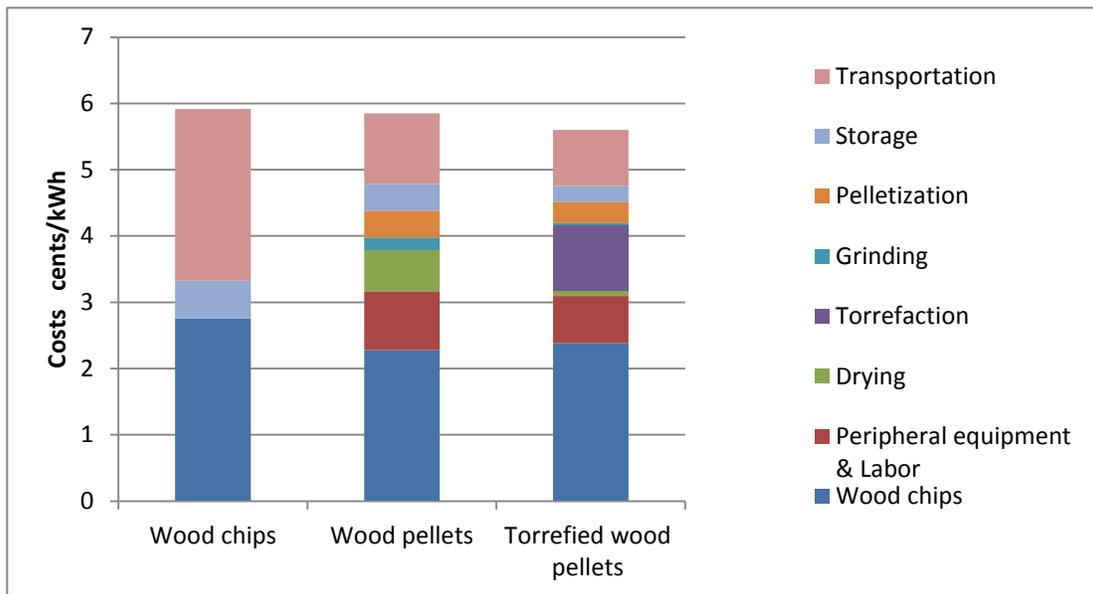
**Figure B2.1.** Cost contribution to electrical power generation from wood chips, wood pellets and torrefied wood pellets when a distance of 300 miles from the RBPD to the power plant is applied. Poplar was used as the feedstock at a biomass cost of \$41.33/dt.
